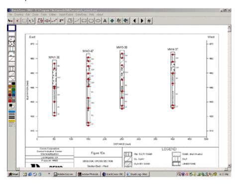
You also have the option of letting the program connect the geological layers using its artificial intelligence:
